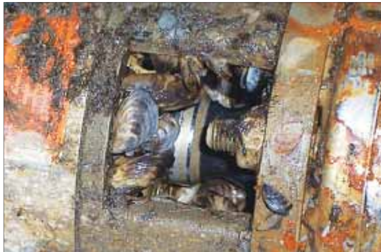
Left: Irrigation systems should see water in mid-April. Above: Zebra mussels, which have moved closer to Idaho each year, clogging a pump (Picture courtesy USDA)
